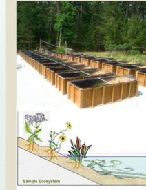
Figure 3. The CEINT mesocosms are large batch reactors exposed to the environment. They have sloped soil beds and are half-filled with water. They are stocked with fish and both an aquatic and a terrestrial species of plant.
