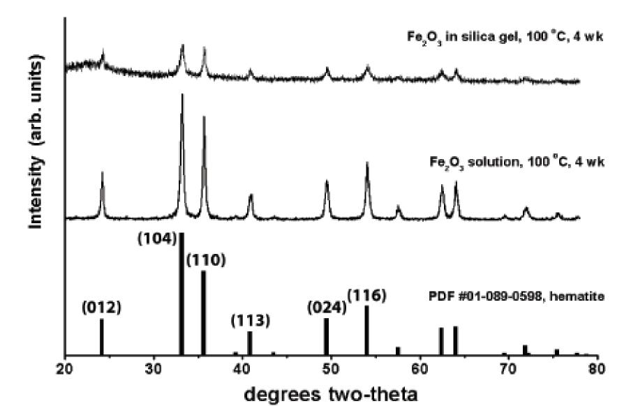
Sherrer analysis of X-ray patterns (shown left) shows both solution and hydrogel grown particles are composed of subunits.
