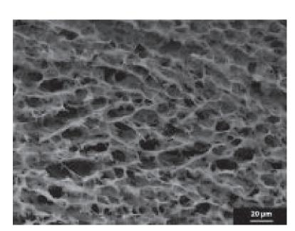
Porous, cellular microstructure of (freeze-dried) silica hydrogel (0.25 M Na<sub>2</sub>SiO<sub>3</sub> and 0.5 M HCl)
