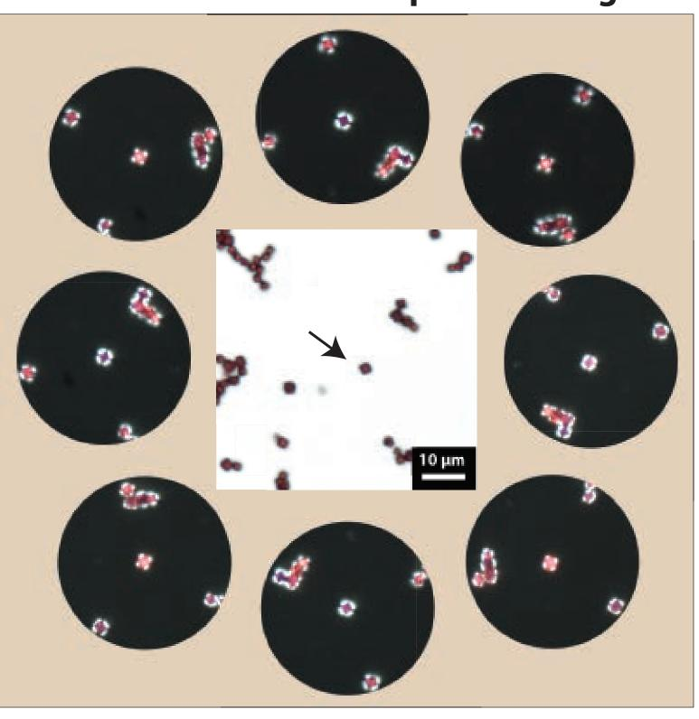
Rotation of both solution (shown above) and hydrogel grown particles under cross polarized light shows both poly and single crystal signatures:
