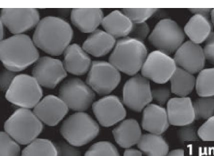
Hematite spheres formed within the gel network Both solution and gel-grown hema-
