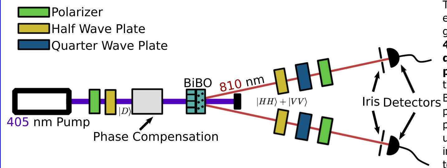
The BiBO crystal used for entangled photon pair generation was pumped with a **405 nm laser.** A block of **quartz was needed for phase compensation** due to the large birefringence of the BiBO. Silicon avalanche photodiode detectors, wave plates and polarizers were set up at the cone opening angle in order to perform a tomography<sup>2</sup> of the state. The waveplates allow us to project any polarization state.
