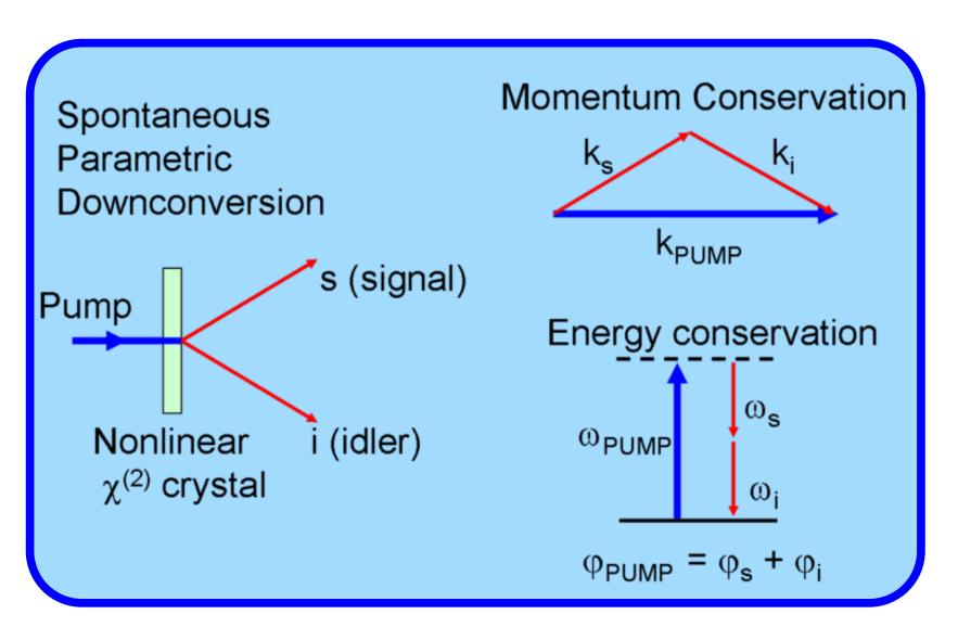
SPDC, with very small probability, will generate entangled photon pairs. BiBO's type-I phase matching ensures the signal and idler polarizations are orthogonal to the pump. Pumping two crystals back to back, with orthogonal principal axes leads to:
