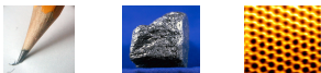
Left: Pencils deposit flakes of multi-layer graphene on paper every time we write (msecc.wisc.edu) Middle: Chunk of graphite (top-gov) Right: AFM image of carbon atom network in graphite (physik.uni-augsburg.de)
